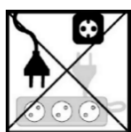
Plug into an extension lead
