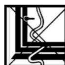
Where the power cable may be damaged
